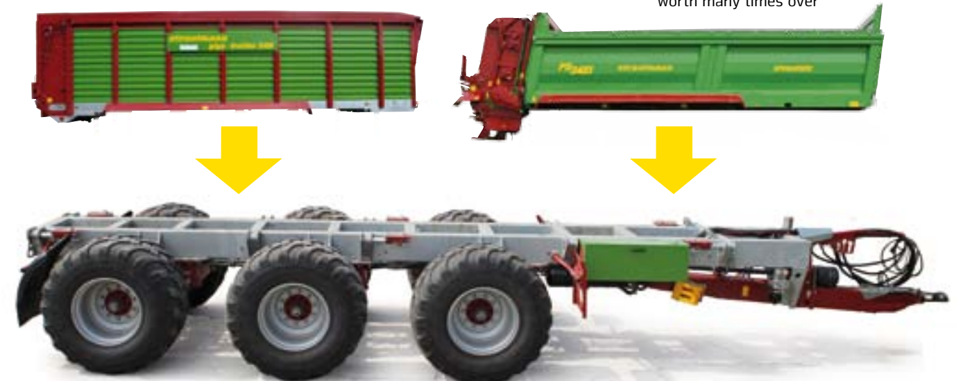
Without use of tools Quick couplings of hydraulic connectors
